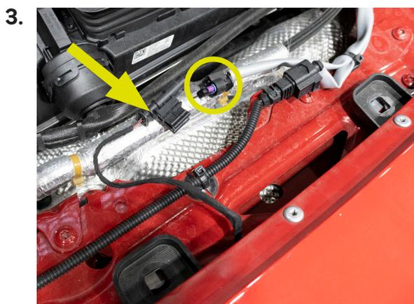
Then loosen the screws of the rear lights, pull them out and disconnect the plug connections. Make sure that no cables are live or trapped.
