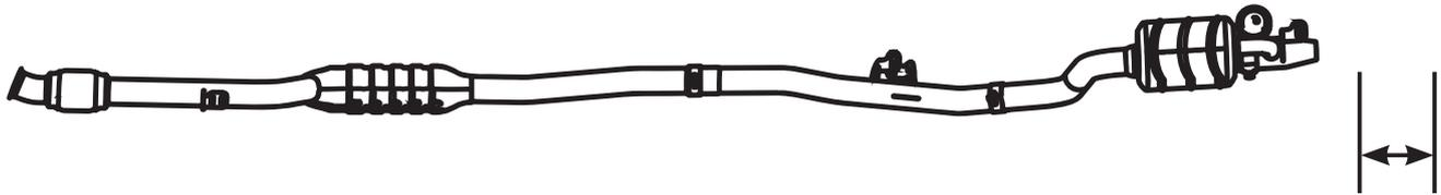
The rubber suspensions, in cold condition, have to be in the right position to give way to the movement towards the rear. It has to be assured, that the whole system keeps sufficient clearance to all parts of the vehicle with and without elongation.
