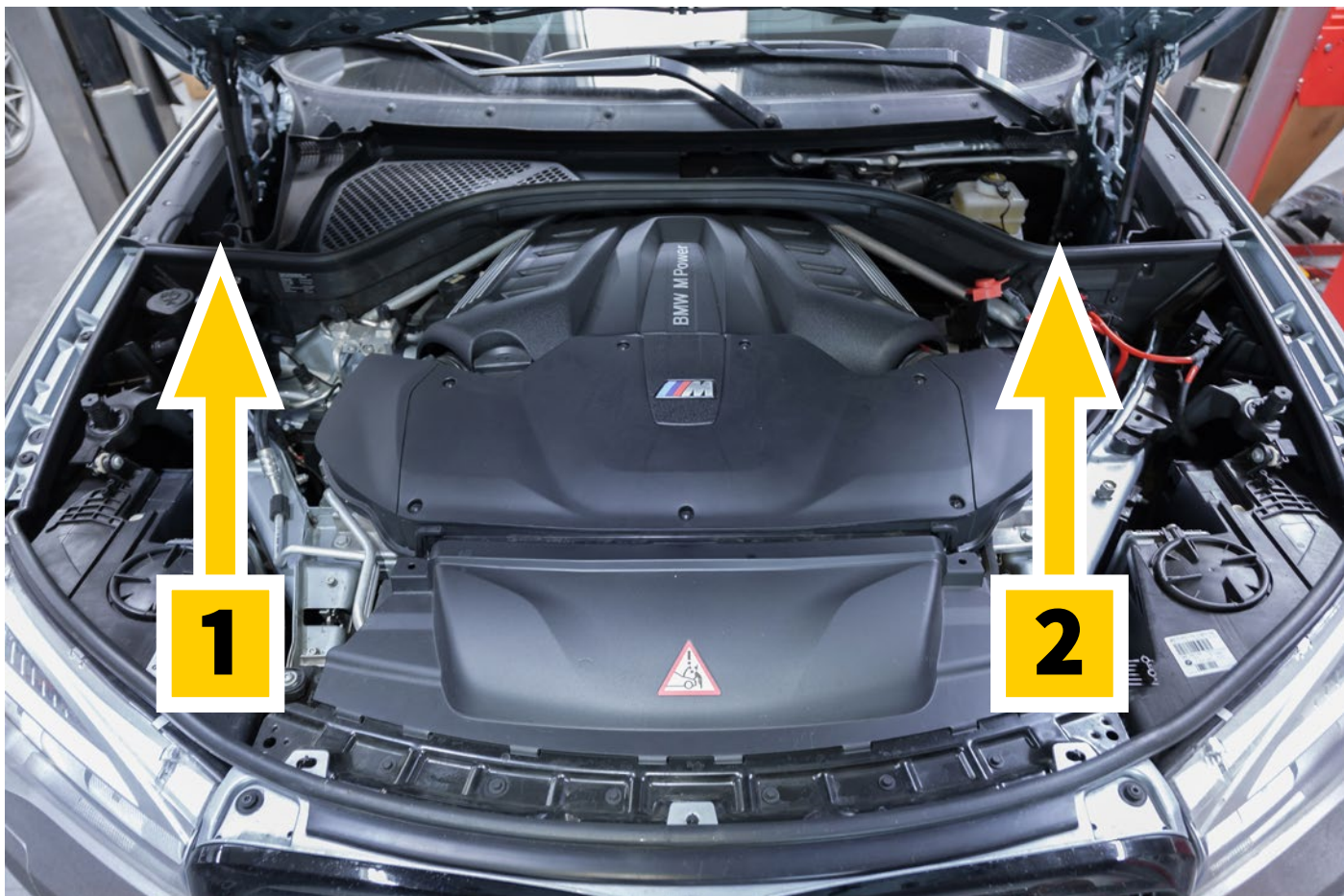
[1] Position der Antenne/position of the antenna eyelet [2] Position von CES-3, Solenoid, Antennenmasse und Vacuumadapter/position of CES-3, solenoid, antenna's ground and vacuum adapter
