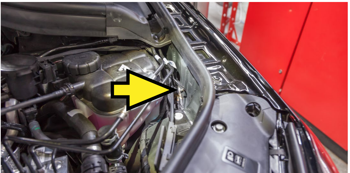
CES-3 Antenne langes, schwarzes Kabel an Masse/antenna long, black cable to ground
